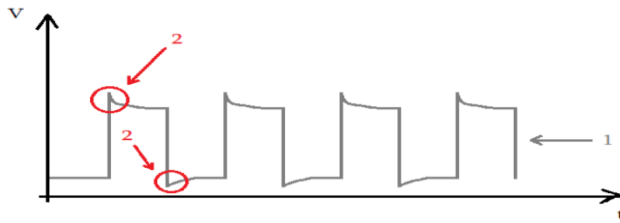
Fig. 1. The periodic signal with noises at its switching moments (1-signal, 2-noises)
