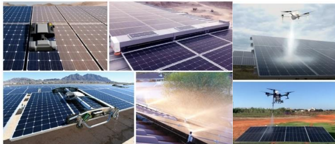
Fig. 5. Automated surface cleaning of solar PV modules: cleaning robots, drones and automated water systems
