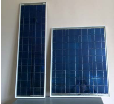
Fig. 5. PV modules prepared with the use of a new encapsulant
