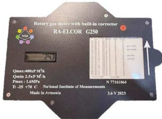
Fig. 3. RA ELCOR (G16 – G400) rotary flow meter screens
