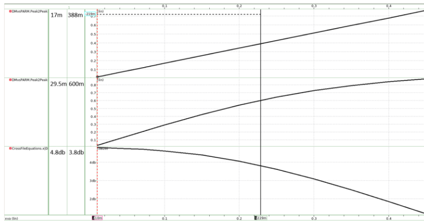
Fig. 7. The waveform showing the improved 1db compression point
